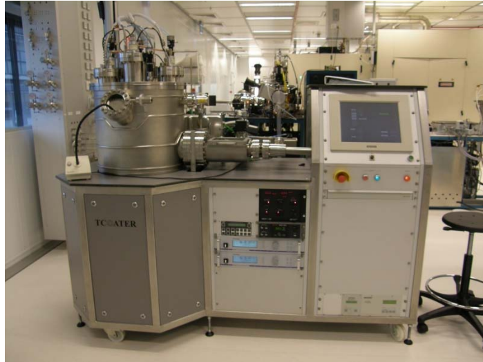
TCOater system which allows sputter deposition of various materials
