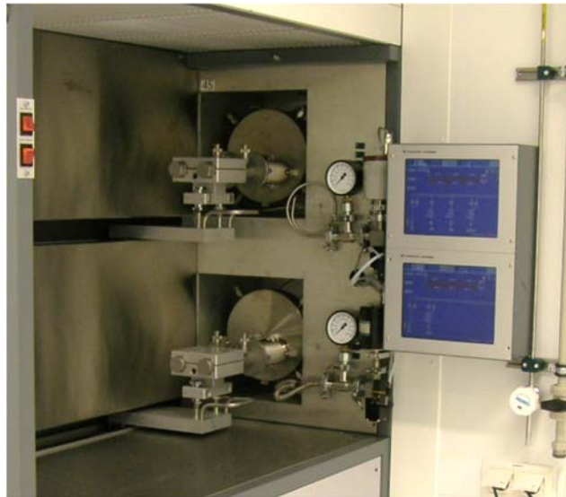
Furnace system for the growth of a CVD layer at high temperature
