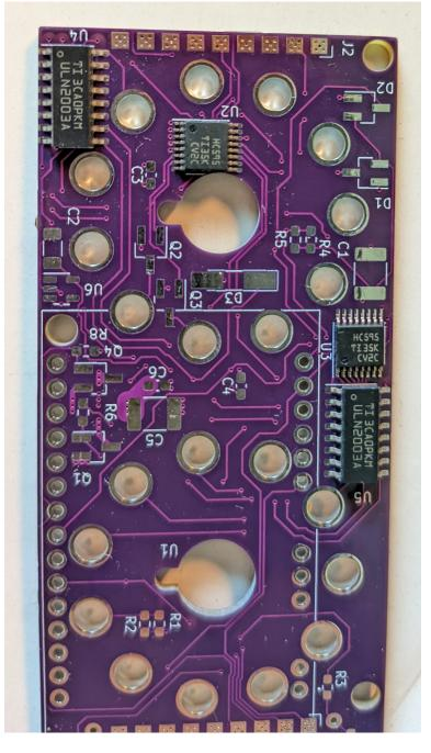
3) Solder the resistors next, R1 through R5 are black with white text, and R6 and R8 are green with white text. For the black resistors make sure to use the resistors with the correct marking, as seen below ("18D" for R3 and "433" for R1, R2, R4 and R5):
