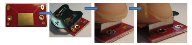
Press the battery holder so the legs bend into the holes. Flip the circuit board. Make sure that metal plate is below the text of the print. Solder the battery holder in place.
