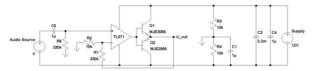
This RC high pass filter has its cutoff frequency at 0.5Hz, so it has minimal influence on the audible spectrum. The resistor has a high enough resistance to be a load to the virtual ground, which is not stable with low impedance loads
