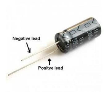
Figure 6.2: Elco pin layout
