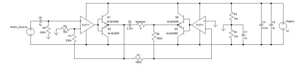
Notice the added right half is an inverting amplifier with an amplification factor of -1, its input signal at the output of the left amplifier (left of C1) and its feedback point at the output of the right amplifier (right of
