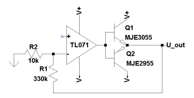
This push-pull pair consist of two transistors, which together form another amplification stage with an amplification factor of 1. This amplification is not really linear, but shows switching characteristics on each flank, but due to the feedback point after this stage, the operational amplifier corrects all these effects.
