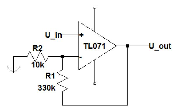
When you solder the final amplifier (not this one above!), use an IC socket for this operational amplifier and be sure to check the datasheet for the pin layout. We can now add anything directly after the operational amplifier; the operational amplifier will make sure the voltage on its input terminals is equal, so the amplification before the resistors is always  $34*U_{in}$ .
