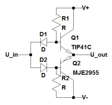
There is another downside to this circuit. To start with, the amplifier will draw a significant current, even in rest. When the diodes badly match the transistors, this current may become as high as several amperes. Furthermore, due to the voltage over R7 and R1, the output swing over the speaker is decreased. When this amplifier is powered at a low voltage, this will greatly influence the volume the amplifier is able to produce. You can correct this by increasing the supply voltage.
