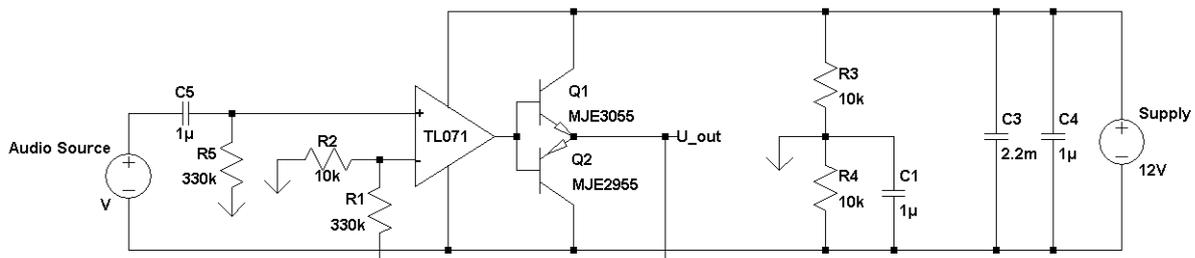
This RC high pass filter has its cutoff frequency at 0.5Hz, so it has minimal influence on the audible spectrum. The resistor has a high enough resistance to be a load to the virtual ground, which is not stable with low impedance loads
