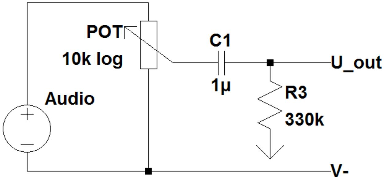
the amplifier a variable gain. It is also possible to swap R1 in the basic design for a potentiometer of the same value. This will keep your input impedance high, but your amplification range will be adjustable from 1 to 34.
