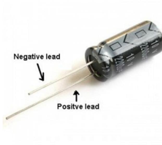
Figure 6.2: Elco pin layout
