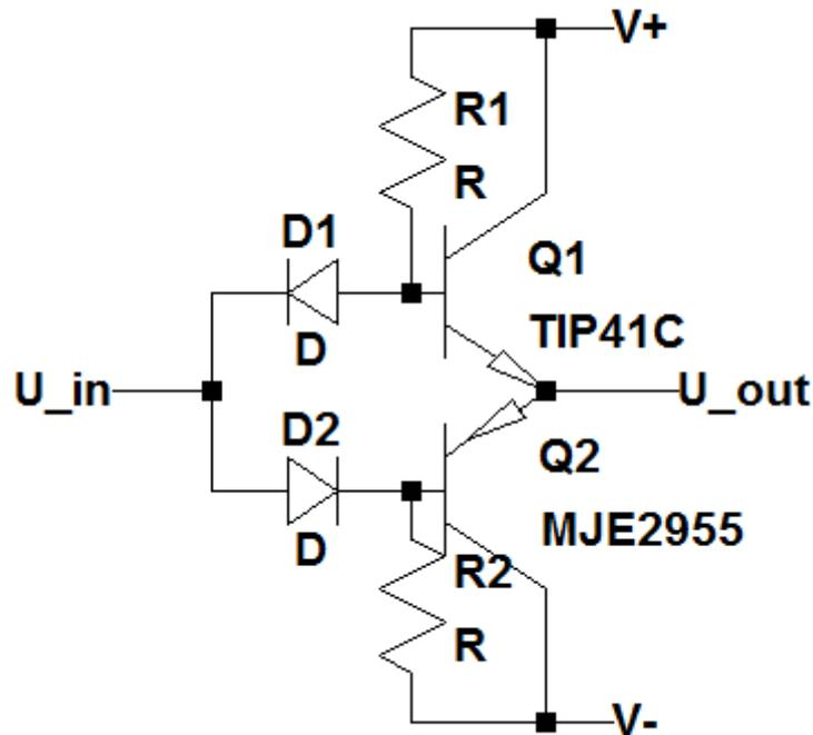
There is another downside to this circuit. To start with, the amplifier will draw a significant current, even in rest. When the diodes badly match the transistors, this current may become as high as several amperes. Furthermore, due to the voltage over R7 and R1, the output swing over the speaker is decreased. When this amplifier is powered at a low voltage, this will greatly influence the volume the amplifier is able to produce. You can correct this by increasing the supply voltage.
