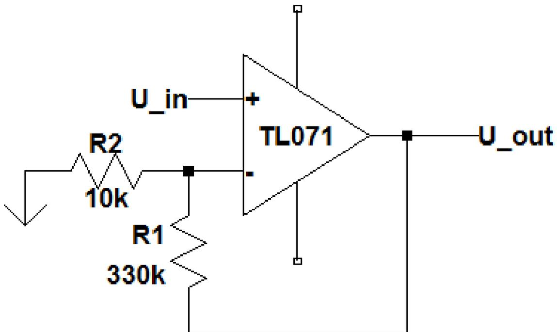
When you solder the final amplifier (not this one above!), use an IC socket for this operational amplifier and be sure to check the datasheet for the pin layout. We can now add anything directly after the operational amplifier; the operational amplifier will make sure the voltage on its input terminals is equal, so the amplification before the resistors is always  $34 * U_{in}$ .
