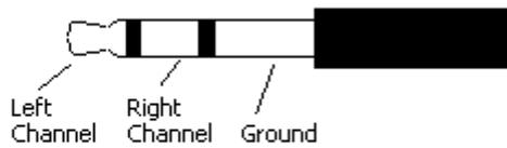
**Connection diagram for standard stereo headphone plug**
