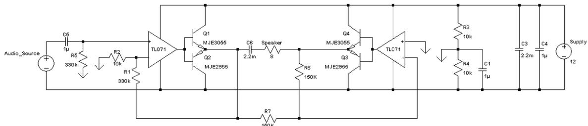
Notice the added right half is an inverting amplifier with an amplification factor of -1, its input signal at the output of the left amplifier (left of C1) and its feedback point at the output of the right amplifier (right of
