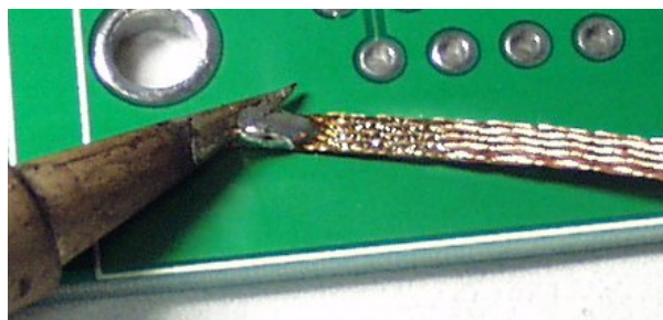
Figure 8.1: How to use a solder wick
